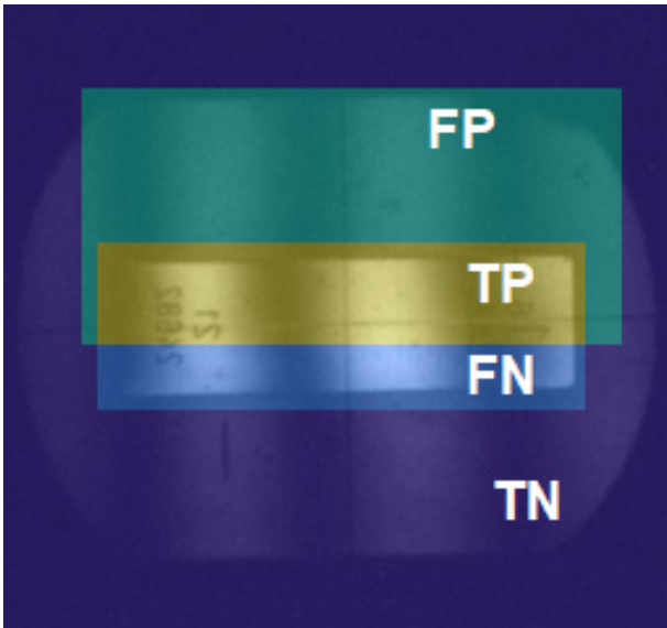
Fig. 8. Example result of detection of the sample object as ROI. Each pixel in the image is categorized to be in one of the four conditions: True positive, true negative, false positive, and false negative.
